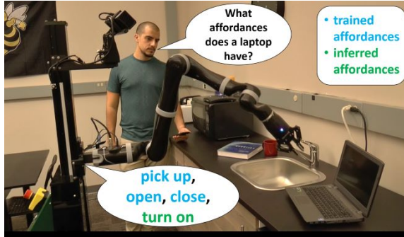
Figure 4.1: RoboCSE can be queried by a robot to infer knowledge and make decisions.
