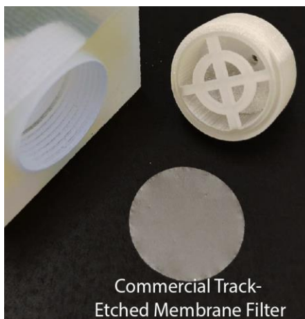
Figure 23: A photo of the 3D-printed device with the filter holder.
