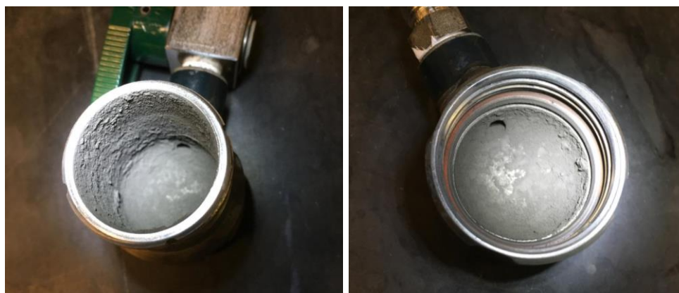
Figure C4: Photos of the milling vessel after reaction with the Ti powder caked on the walls of the vessel.
