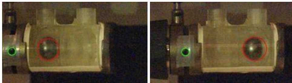
Figure 15: Frames representing the two dominant collisions in the reactor; backwards (right) and forwards (left). Image identification of the ball (red) and mill position (green) and highlighted as well.
