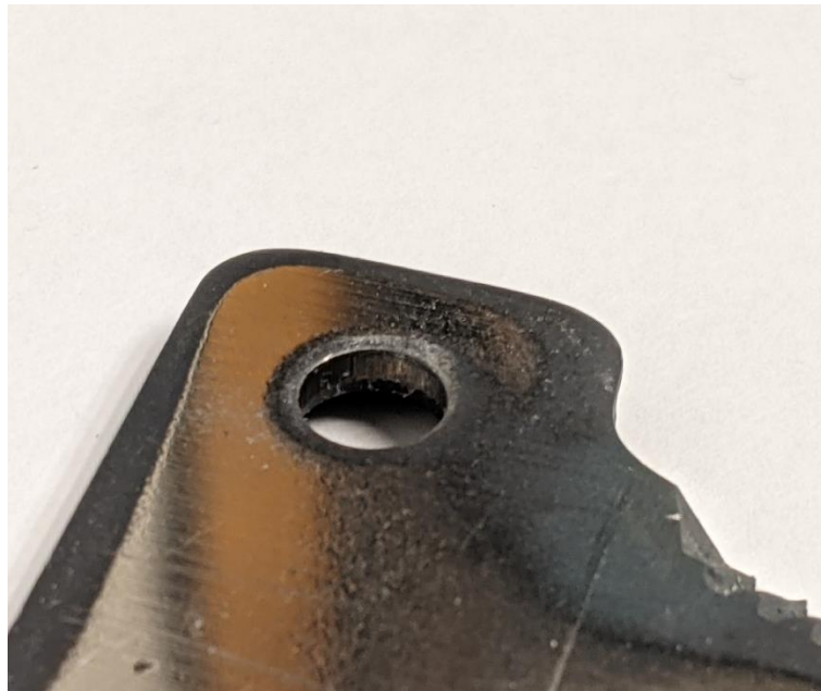
Figure 64: Piercing witness marks on inside of mounting holes
