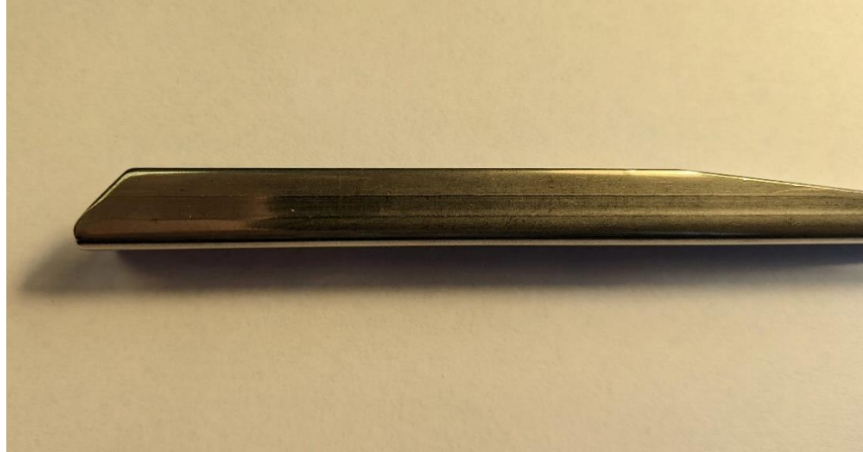
Figure 16: Rice transplanter claw side view showing the metal finish difference along the center
