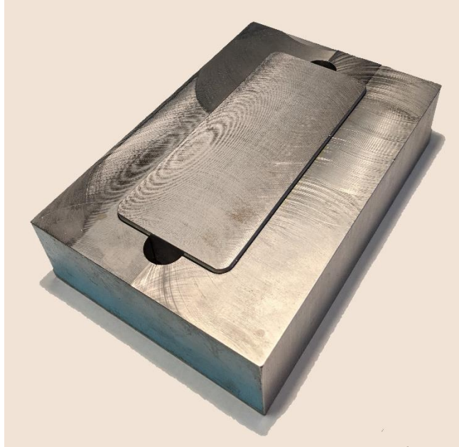
Figure 35: Assembled machined rice transplanter claw bending punch and die set
