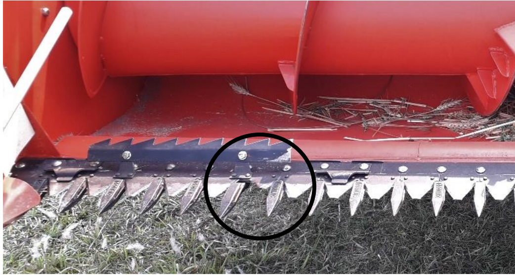
Figure 52: Full-feed combine harvester cutter bar with broken blade
