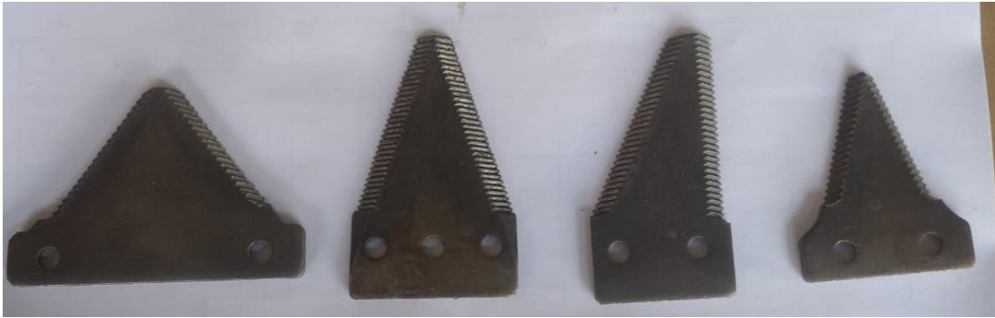
Figure 55: Spare half feed combine harvester blades in Bangladesh. From Left to Right: large bottom blade, top blade, half blade, and small bottom blade
