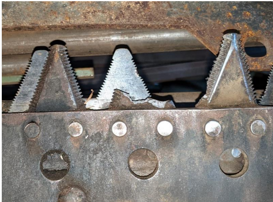
Figure 53: Half-feed combine harvester cutter bar with broken blade
