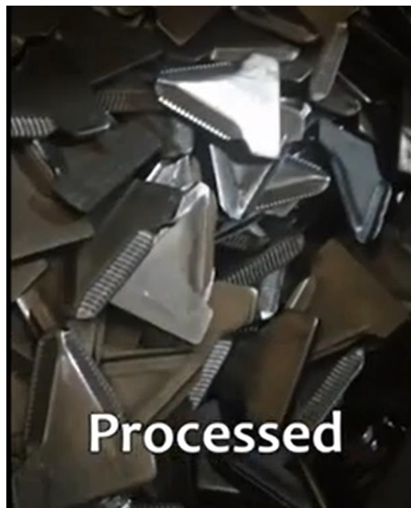
Figure 60: Post serrated edge forging combine harvester blades
