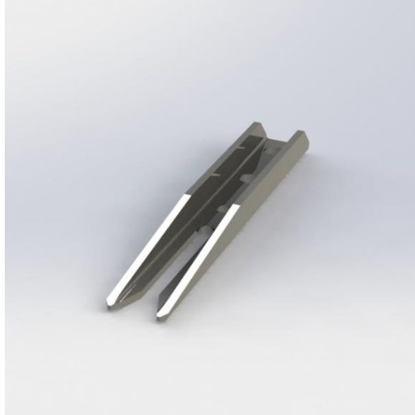
Figure 24: SolidWorks rendering of rice transplanter claw
