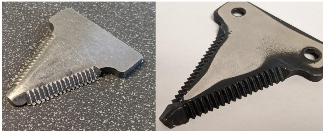
Figure 99: Comparison of test blade and original half-feed combine harvester small bottom blade
