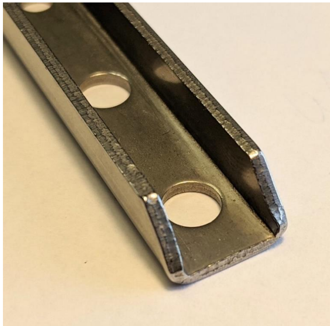
Figure 14: Piercing witness marks on inside of mounting holes
