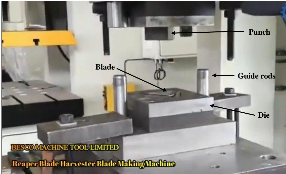
Figure 57: BESCO combine harvester blade serrated edge forging punch and die set
