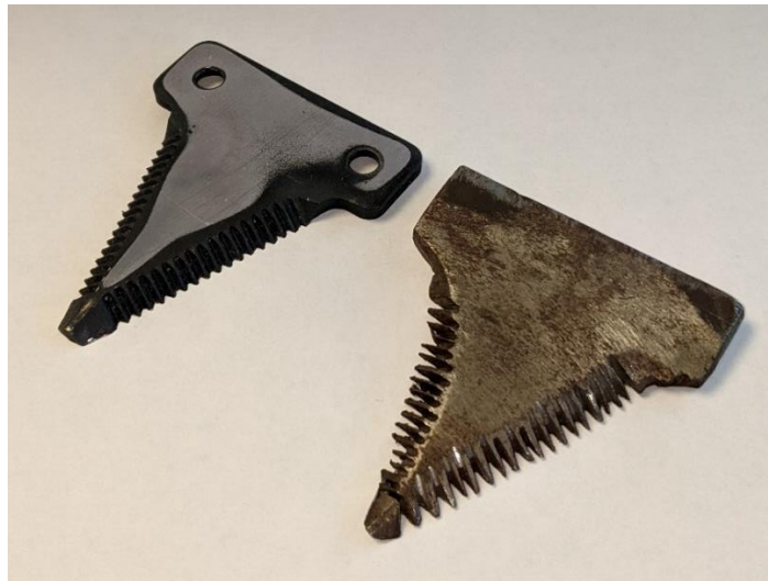
Figure 54: Original combine harvester blade (left); NRE manufactured combine harvester blade (right)
