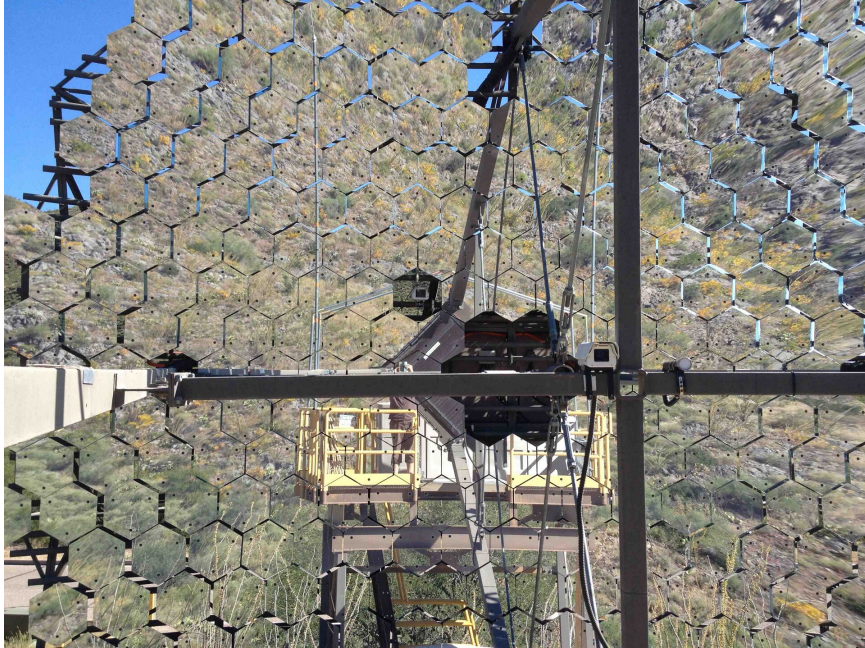
Figure 4.4: A picture showing the dedicated camera mounted on the OSS of one of the VERITAS telescopes. From the VERITAS internal wiki page for Optical Reflectivity.
