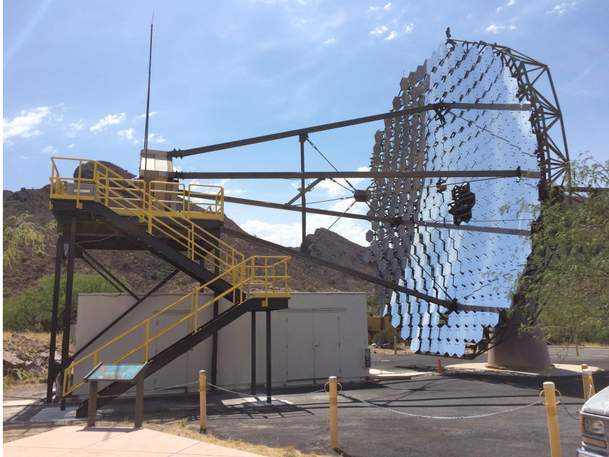
Figure 4.3: A photo showing one of the VERITAS telescopes. The profiles of the profile of the camera housing along with the reflector can be seen. Also shown is the trailer that contains the necessary electronics and computing equipment specific to each telescope.
