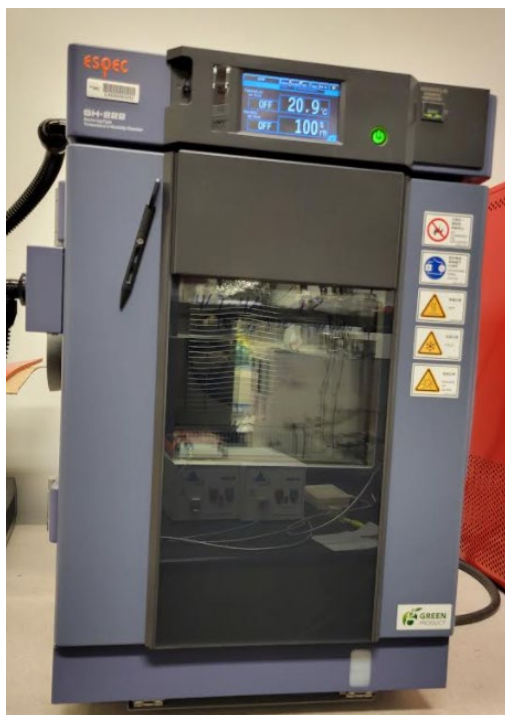
Figure 24 Photograph of the experimental setup for in-situ transmission measurements as humidity in the chamber was cycled between 55 and 95% RH
