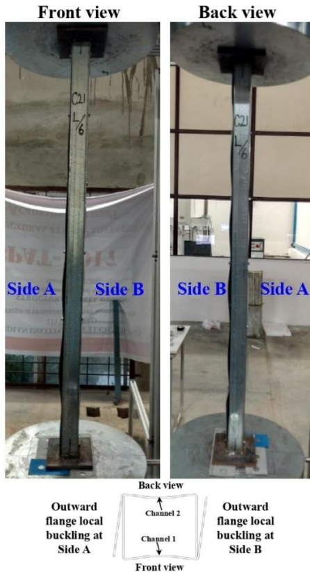
Fig. 4. Local buckling Failure mode pattern in face-to-face connected built-up columns
