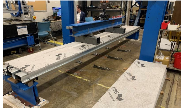
Figure 8: Four-point bending test
