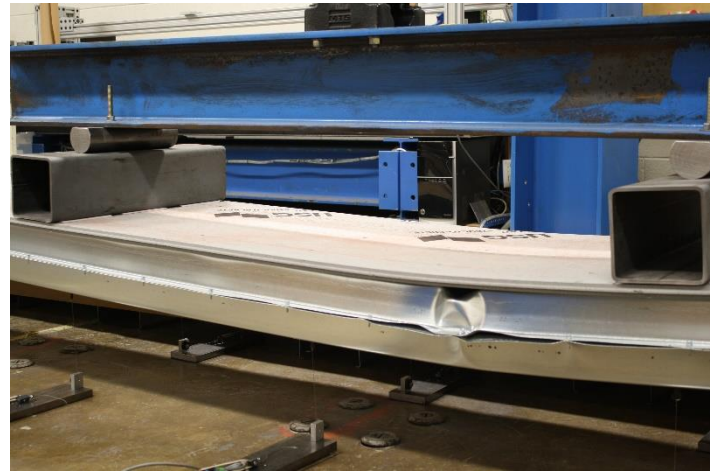
Figure 13: Local buckling and plastic mechanisms in the bottom and top deck
