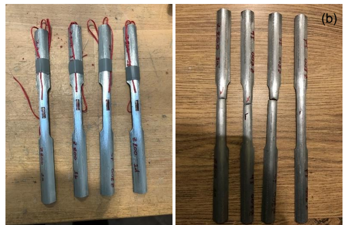
Figure 4: Typical curved specimens wired cutting from the section, Z-W200T2.0 and specimens extracted from curved locations 1a, 1b, 1c, 1d and the associated gripped inserts (a), and the test specimens before and after testing with attached strain gauges (b).
