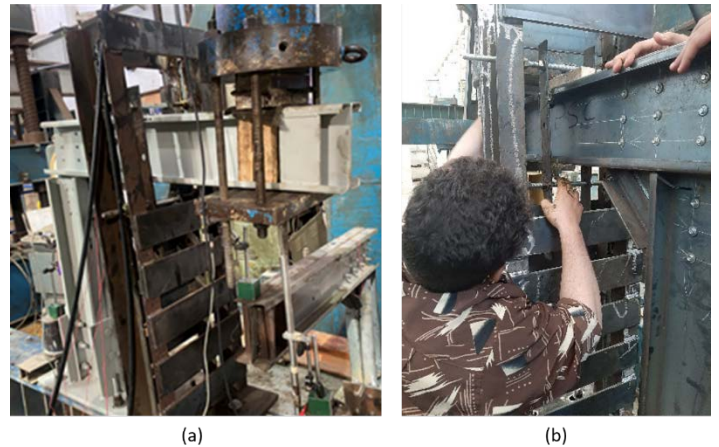
Figure 5: (a)Steel lateral support (b)lubrication between the support and flange plates
