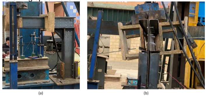
Figure 6: Pilot Specimen (PS) (a) Configuration and testing (b) Deformed shape of PS
