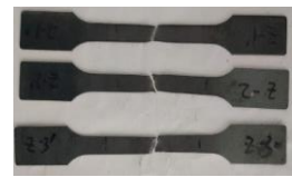
Figure 4: Specimens after tensile fracture cut from the flat plate
