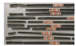
Figure 5: Specimens after failure cut from the corner area
