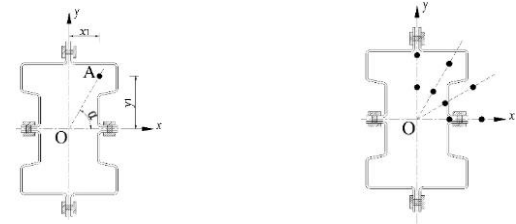
(a) Load point positioning parameters (b) Load Point Distribution Figure 8: Load point positioning parameters and distribution map
