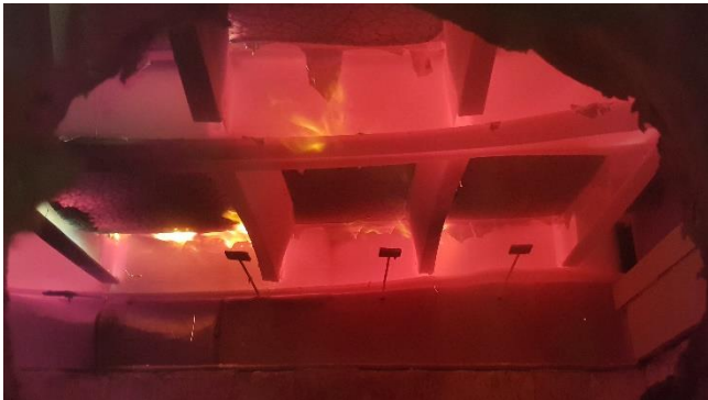
Figure 26: Test specimen of configuration A after 30 minutes of fire
