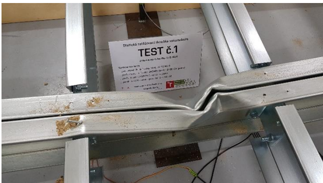
Figure 17: Progressed failure mode of middle double primary beam
