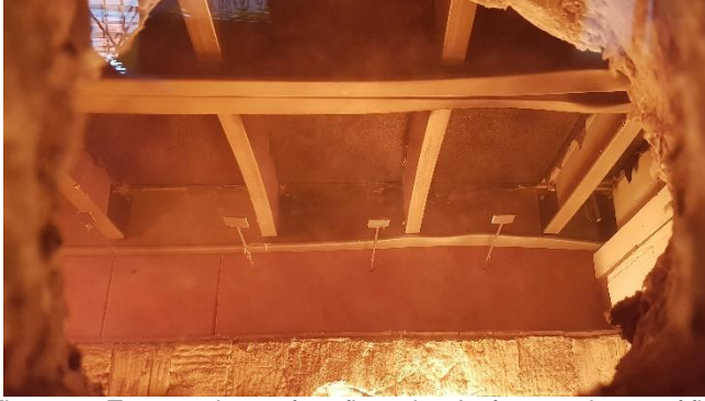
Figure 25: Test specimen of configuration A after 23 minutes of fire
