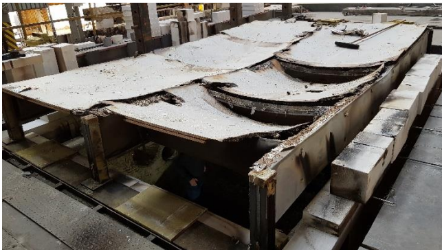
Figure 27: Test specimen of config. A after burning and extinction
