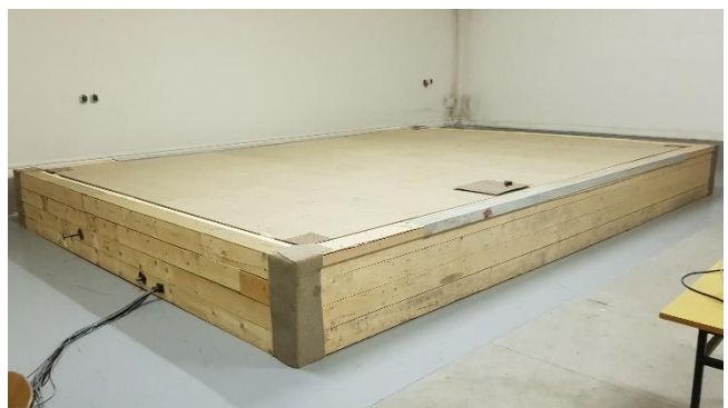
Figure 7: Test specimen with installed chipboards
