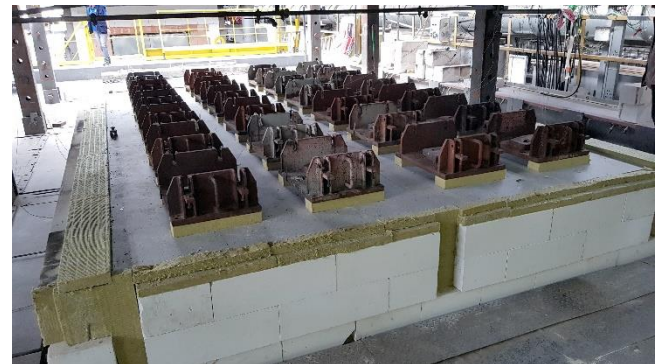
Figure 24: Applied load on test specimen (configuration A)
