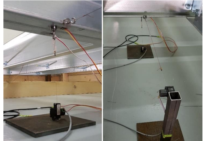
Figure 10: Potentiometric sensors for measuring vertical and horizontal deflections at the beam mid-spans
