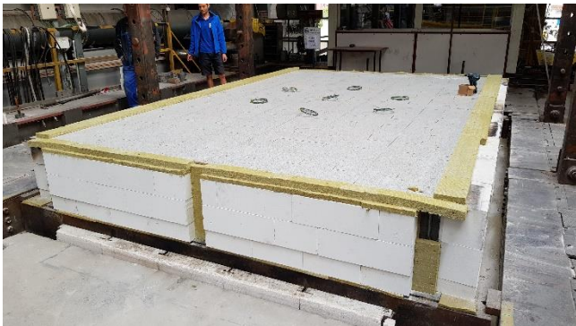
Figure 22: Test specimen (configuration A) seated on the furnace
