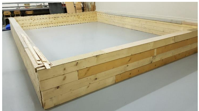
Figure 5: Wooden box standing on reinforced concrete floor slab
