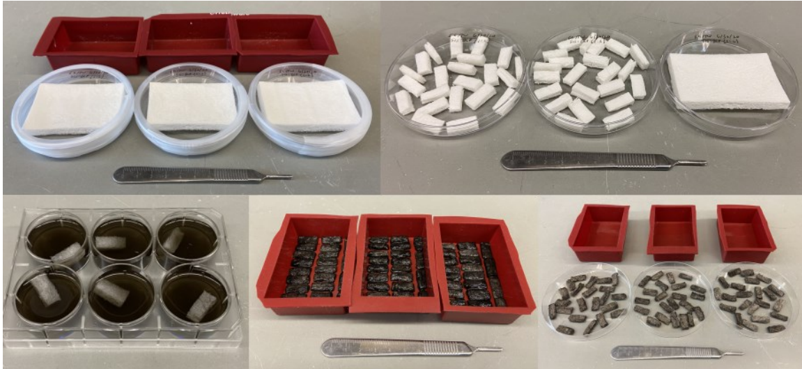
Figure 3.3: The biomimetic mixture was lyophilized, yielding a white, porous biomimetic bone graft material (upper left), which was then cut into pieces (upper right) for implantation in a rat model of spinal fusion. The pieces were instilled with polydopamine via immersion in a dopamine solution (lower left), washed with distilled water to remove excess dopamine molecules (lower middle), and then lyophilized to yield porous, homogenously dispersed solid mixtures of ECM and calcium phosphates instilled with polydopamine, called BioMim-PDA (lower right).
