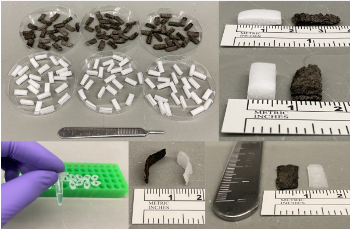
Figure 3.4: Implant-sized pieces of BioMim-PDA (black) and collagen (white) are shown for comparison. The dry dimensions of all implants were 15mm×5mm (length×width). rhBMP-2 (0.2µg, 2.0µg, or 20µg) in aqueous solution (lower left) was uniformly distributed onto BioMim-PDA or collagen sponge, and the wetted graft was allowed to stand for 15 minutes before implantation; the wetted grafts assumed nearly identical physical dimensions (lower middle and lower right) and handleability.
