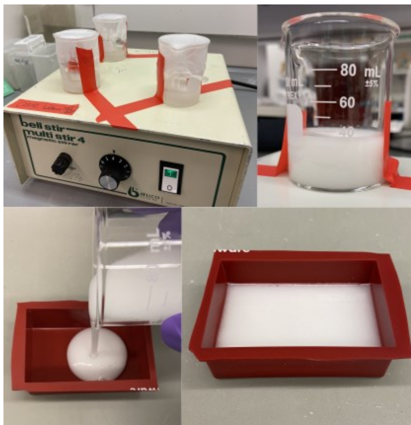
Figure 3.2: The SIS was enzymatically digested using pepsin in a dilute HCl solution for 24 hours on a magnetic stir plate (upper left), and then neutralized with dilute NaOH. Afterwards, an 80:20 biphasic mixture of beta-tricalcium phosphate and hydroxyapatite was homogenously incorporated with stirring (upper right), and the biomimetic mixture was then poured into a 2”×3” mold (lower left and lower right) and incubated at 37 °C.
