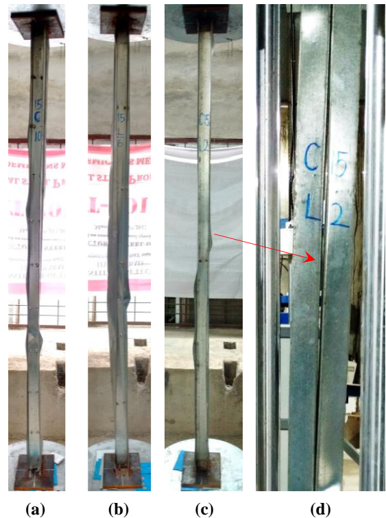
Fig. 2. Failure modes of 50/100-1800 set specimens: (a) 50/100-1800-L/10 specimen; (b) 50/100-1800-L/6 specimen; (c) 50/100-1800-L/2 specimen; (d) 50/100-1800-L/2 specimen-separation failure;
