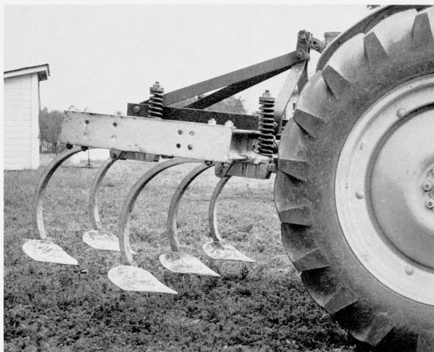
Heavy field cultivator (equipped with "moldboard" shovels) as used in the mulch tillage experiments.
