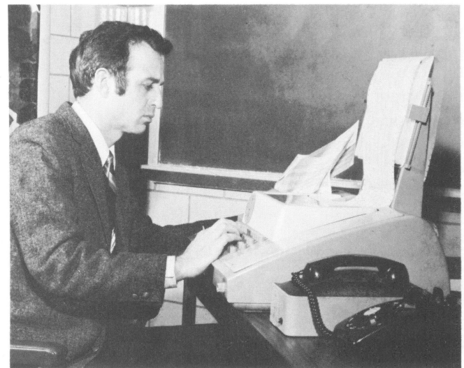
A computer terminal, tied to a central computer by telephone, enables researchers to forecast costs of producing and marketing agricultural products.
