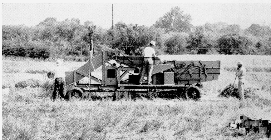
Equipment such as this was used by Station agricultural engineers to evaluate the grain losses from the combine. Some combines vary in their ability to handle high moisture straw.
