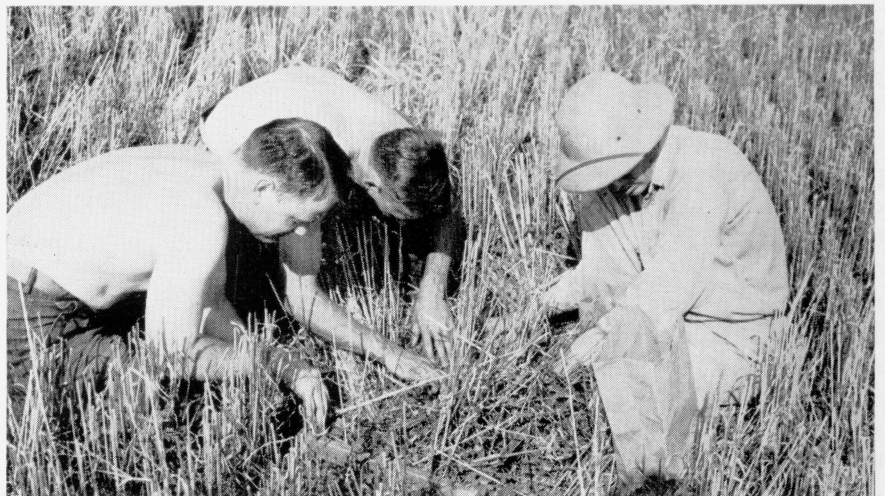
Agricultural engineers evaluated cutterbar loss by spot checking and counting fallen kernels.
