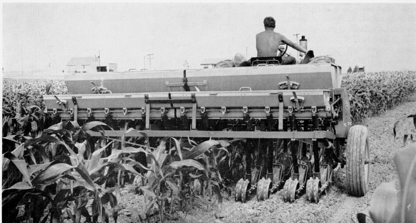
The machine pictured here is one of the first experimental type band seeding drills manufactured by the Brillion Iron Works. Components may be removed to allow adapting to various row widths.
