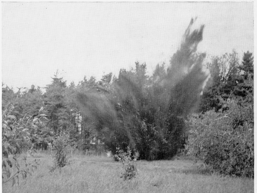
The Station photographer snapped this picture just as the 2.7 pound charge of dynamite was being set off. Top and lateral branches had previously been removed.
