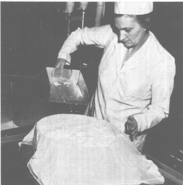
Soft White cheese curd is collected in cloth-lined hoop by Mrs. Natalija Kapac, University of Skopje, Yugoslavia. For the manufacture of White cheese, the rennet coagulated curd is placed directly in a cloth-lined hoop without prior cutting and cooking.
