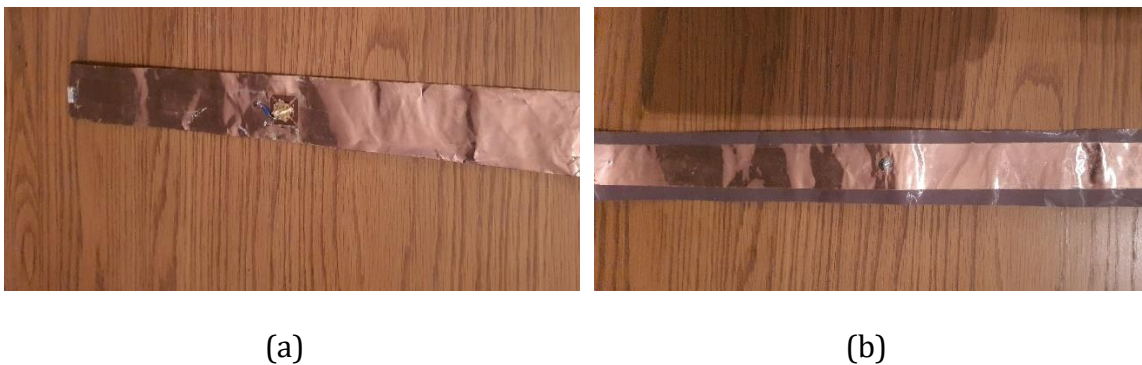
Figure 6.18: D-dot section chemically etched onto Pyralux ® flexible substrate (a) etched Shield side with SMA connector (b) etched electrode side.
