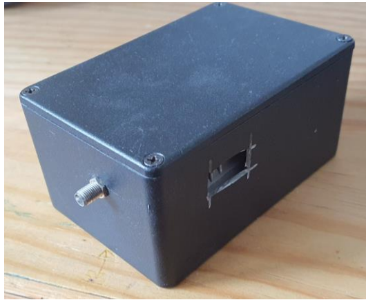
Figure 6.28: Fibre optic transmitter in cast aluminium case.
