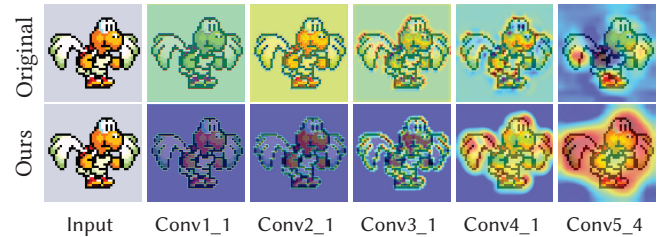
Fig. 9. Class activation maps of original VGG19 pre-trained with ImageNet (top row) and our structure extractor (bottom row). The original VGG19 highlights everywhere with warm colors (especially in the lower convolutional layers), while our extractor can focus on regions of interest and the individual activation point follows a cell structure. The shallow layers of our extractor focus on local regions with activations in smaller cells, and the deeper ones focus more on the global structure. (©Nintendo Co., Ltd.)
