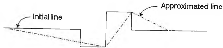
Figure 4.3.2 Effect of a small perturbation on Berthod's line finder
