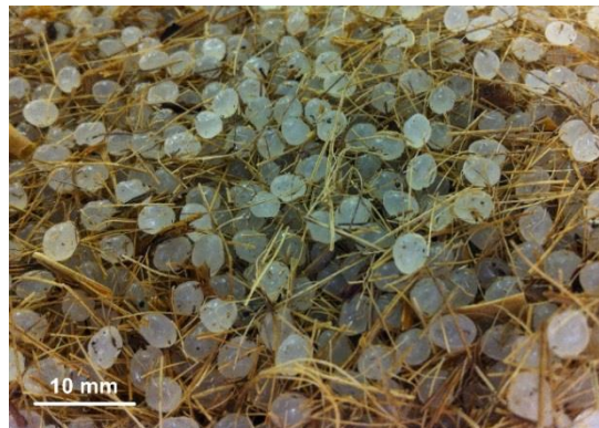
Figure_Apx E-3. Agave tequilana fibres and poly(lactic) acid premixing after compounding.
