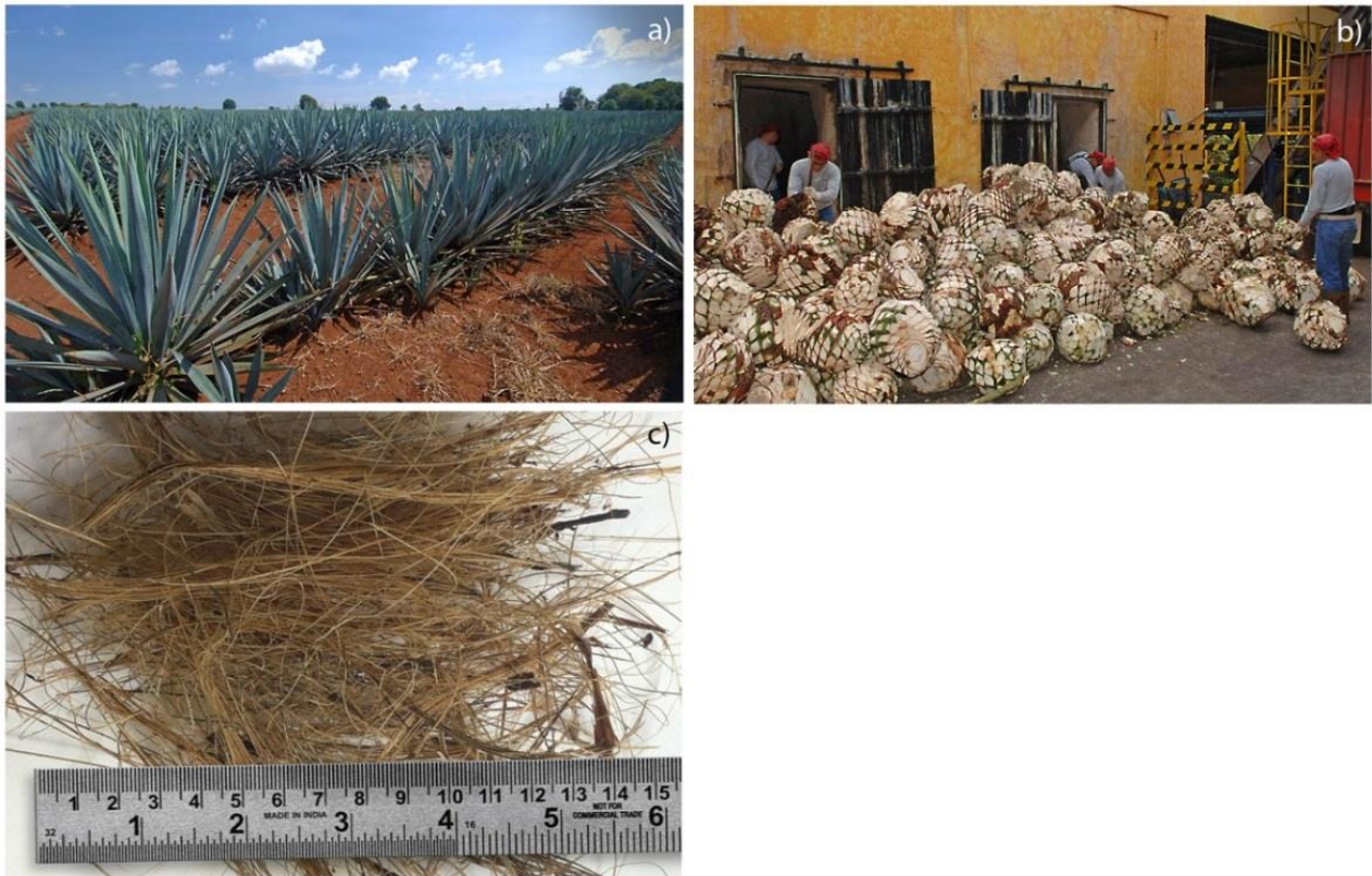
Figure 34. Agave tequilana plant and fibres. a) Agave tequilana plants also known as blue Agave (Needham 2014) [221]. b) Agave tequilana heads are steamed cooked at 90-95 °C for about 18-24 hours [153]. c) Dry bagasse obtained after the heads have been shredded to extract plant juices.
