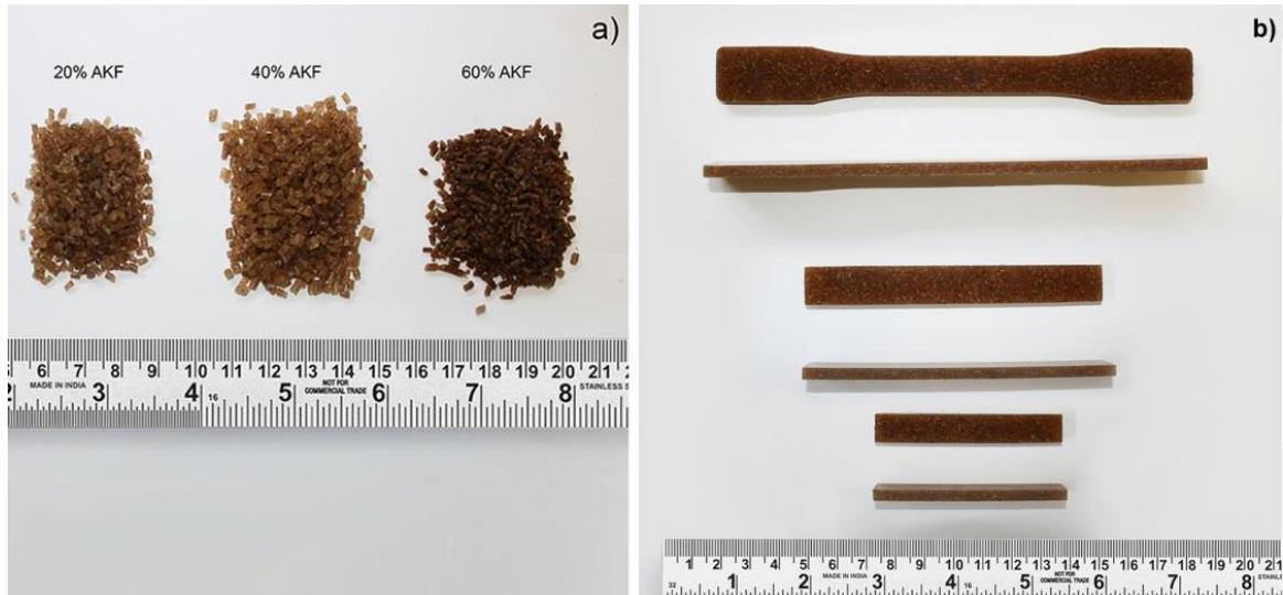
Figure 62. Agave tequilana fibres and poly(lactic) acid bio-based composites specimens. a) Pelletized composites with different fibre volume content. b) 40% (v/w) AKF/PLA composite specimens. Top: Tensile test specimens. Middle: specimens used for three-point flexural bend test. Bottom: specimen used for impact test.
