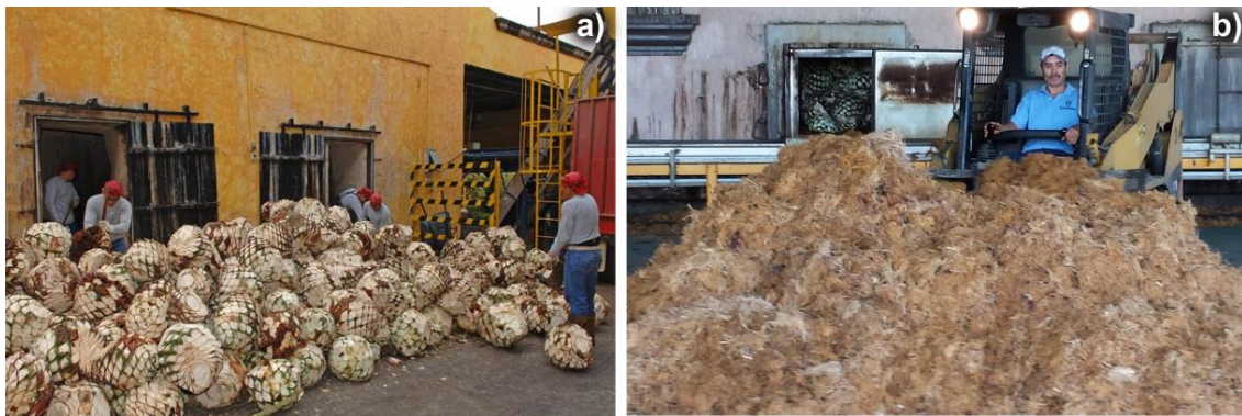
Figure 16. Tequila production stages. a) ATW heads being transported. b) ATW bagasse after milling. Source [153].
