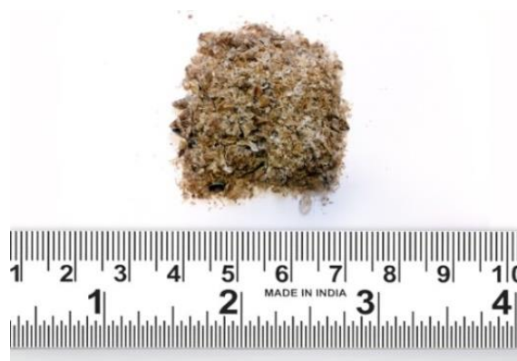
Figure 99. Mechanically treated Agave tequilana fibres and poly(lactic) acid bio-based composite sample ground at 25,000 RPM.
