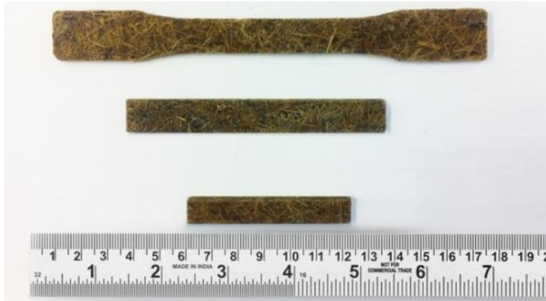
Figure 77. 60% (w/w) Agave tequilana and poly(lactic) acid bio-based composite specimens. Top: specimen used for tensile test. Middle: specimen used for three-point flexural bend test. Bottom: specimen used for impact test.
