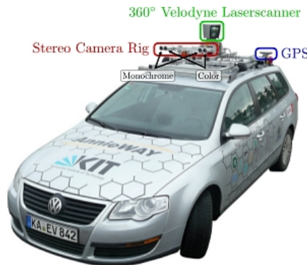
Figure 3.8: Sensor setup used to record the KITTI dataset, extracted from [11].
