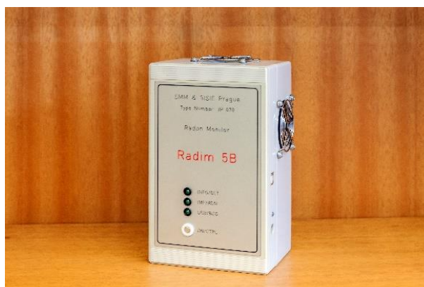
Figure 7.1 - Radim 5B radon monitor
