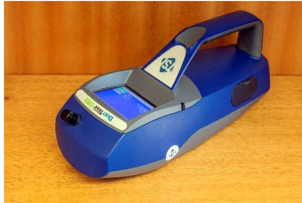
Figure 5.1 - TSI DustTrak DRX 8534 particle monitor
