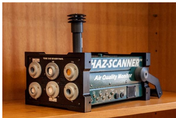
Figure 3.2 - Haz-Scanner IEMS Indoor Environmental Monitoring Station
