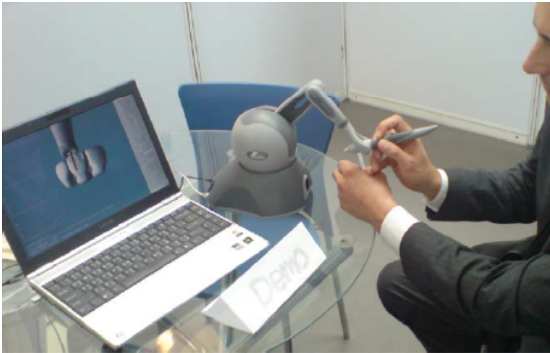
Figure 2.6: PHANTOM arm, retrieved/adapted from [Suebnuarn et al., 2009]
