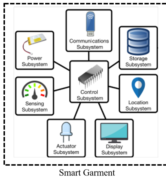
Figure 2.4: Basic structure of an internet of things (IoT) smart garment system [3].
