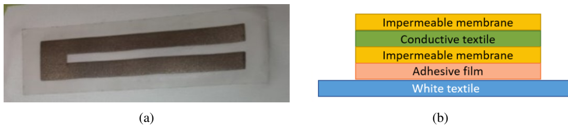
Figure 4.7: UP180+b with impermeable membrane: (a) photo; (b) Structure representation.
