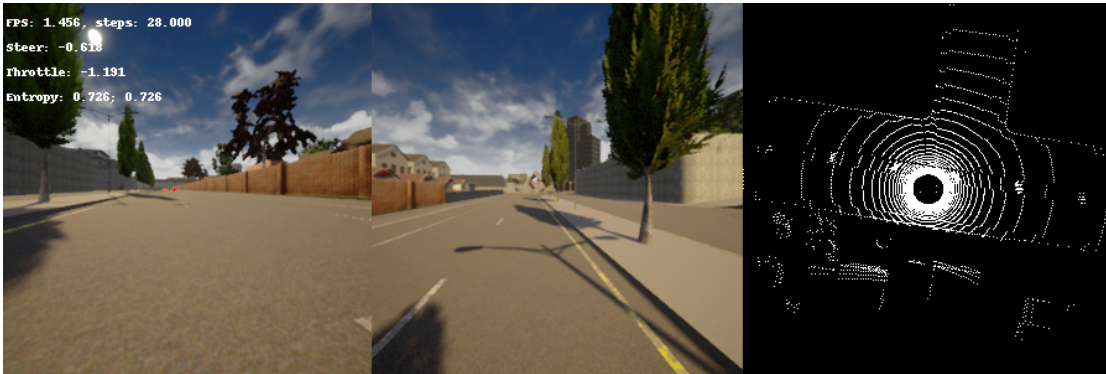
Figure 3.5: Final fused image of the cameras and LIDAR, from left to right, RGB front, RGB Back, LIDAR Projection. Note the text on the left corner is not part of the input.
