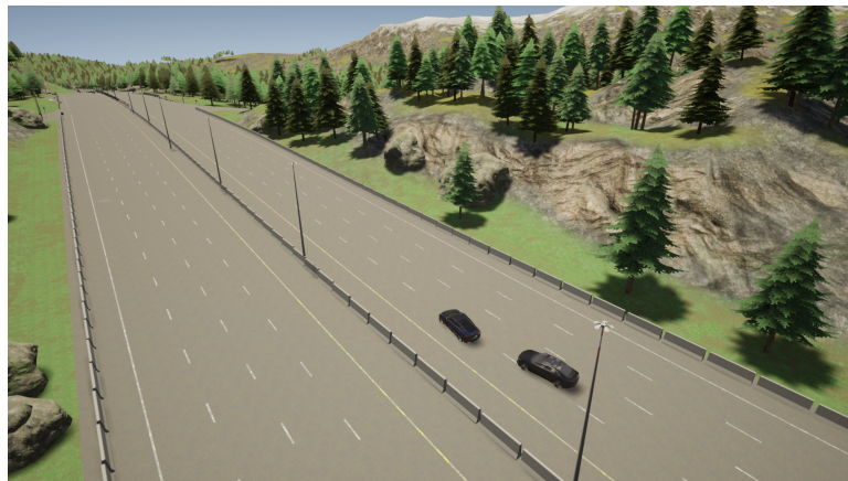
Figure A.5: SAC agent in Cut In scenario. The right most vehicle is the agent and he has to keep in his lane while another vehicle (in the left most lane) cuts in front of him.
