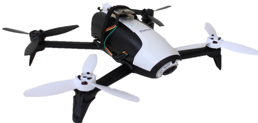
Figure 3.9: ESP32 DevKit integrated into Bebop 2
