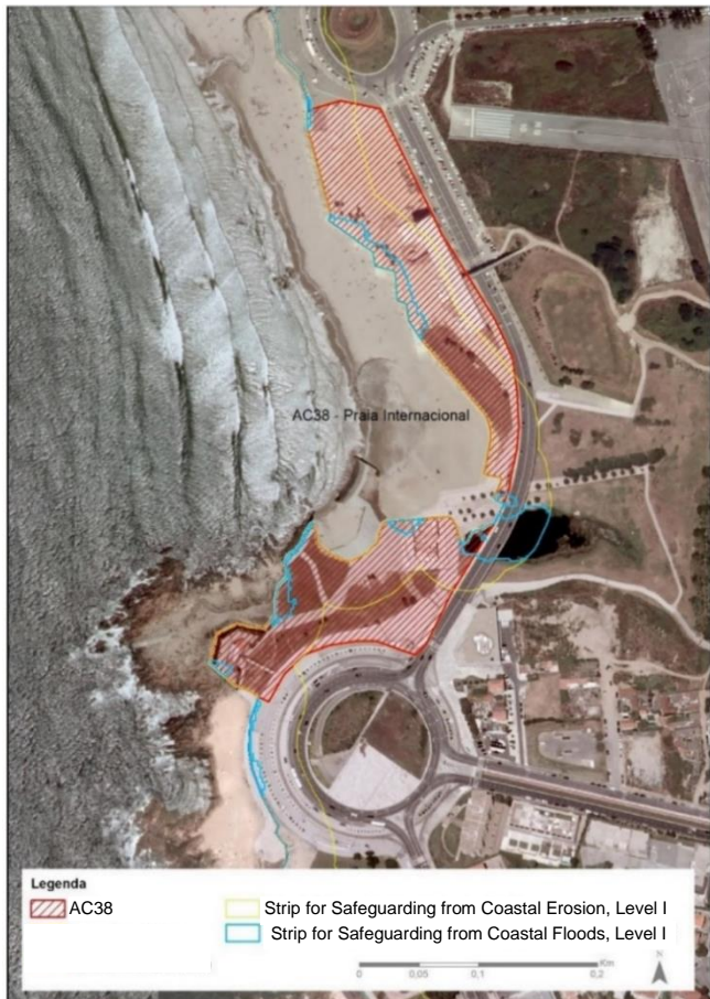
Figure 22 (top left). The Critical Area 38 – Praia Internacional , is partially artificialized and partially located above a rocky platform. The Strip for Safeguarding from Coastal Erosion for 2050 includes almost the entire area located at the west of the roadway ‘Via do Castelo do Queijo’ and the roundabout ‘Praça Gonçalves Zarco’. For this Critical Area, the POC proposes a strategy of Protection , based on the following specific interventions: beach nourishments, construction of a detached breakwater and construction of a rainfall submarine out-flow pipeline (POC-CE 2018 c, p.41).
