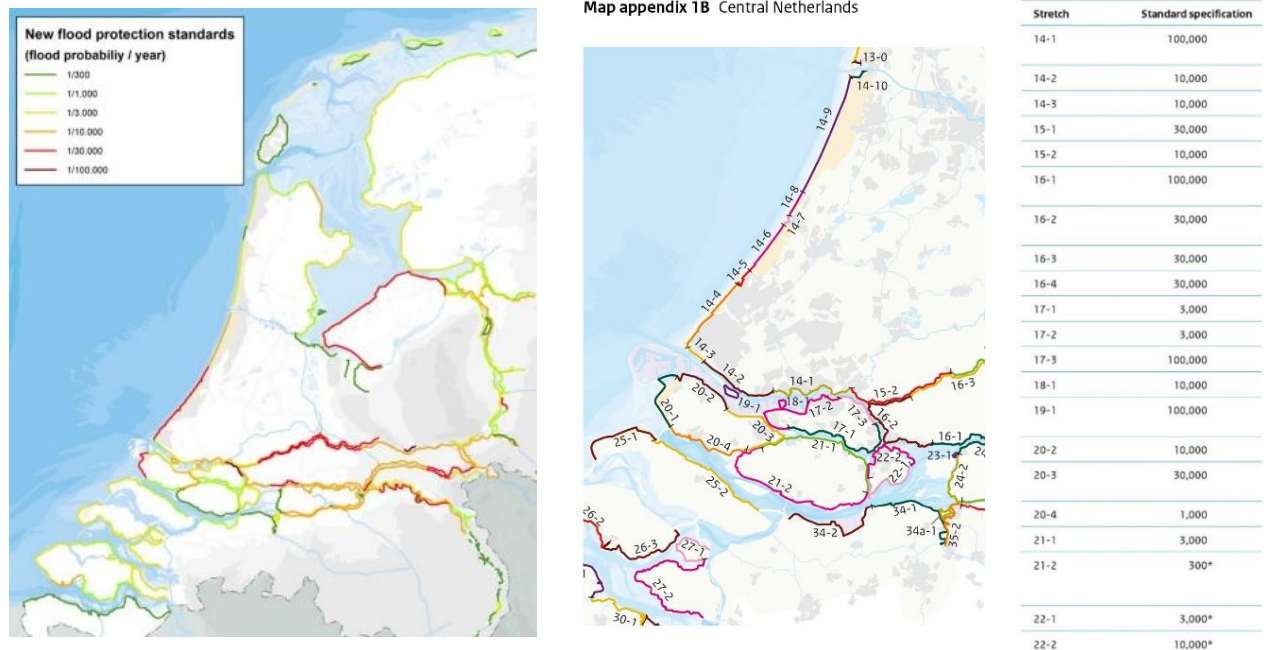
Figure 37 (left). The new flood protection standards, expressed as a flood probability per year , proposed for different sections of flood defences. Source: Alphen 2015; Klijn et al. 2015. Figure 37, right: the proposed 'standard specifications' in a class of flood probability per section of defences (DP 2014, p.158). Three areas required special attention (their standards must be increased): the Rhine Estuary-Drechtsteden, areas around major rivers, and Almere (in Amsterdam); and, in areas where the pre-existing level of protection was satisfactory, it is necessary to maintain and manage the existing defences (DP 2013, p.7).
