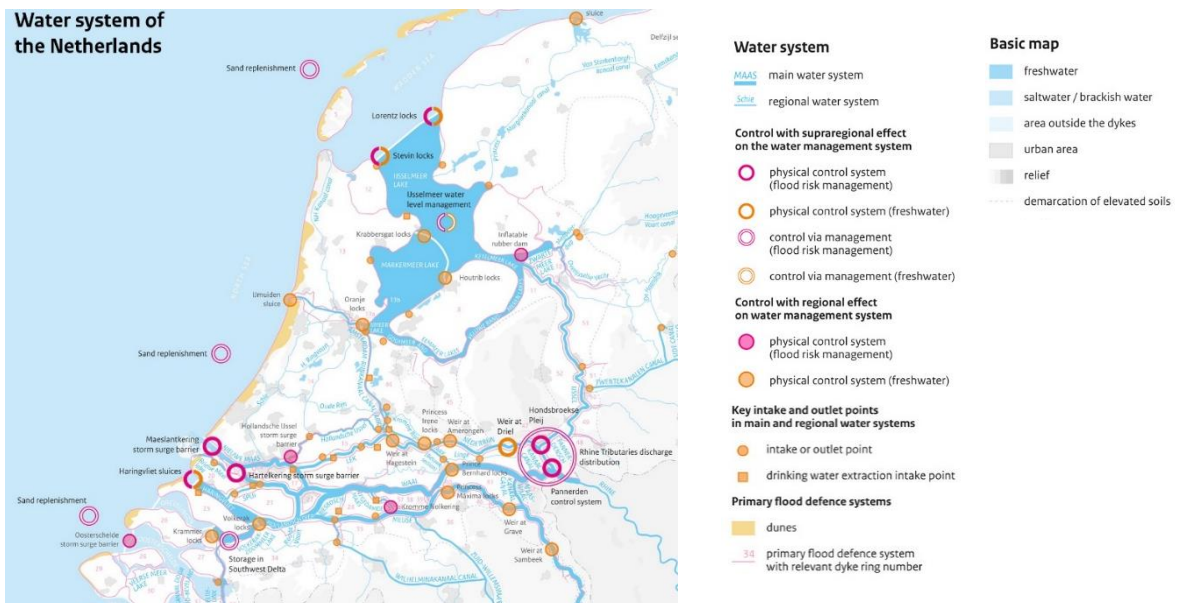
Figure 26. Dutch water system, including the flood risk management (FRM) system and freshwater supply system. The main water system includes (main) ‘primary controls’ and (regional) secondary controls. Source: DP2014, p.151.
