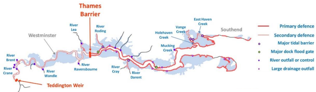
Figure 4. The flood defence system in the Thames Estuary. Source: Ramsbottom and Sheppard 2017.
