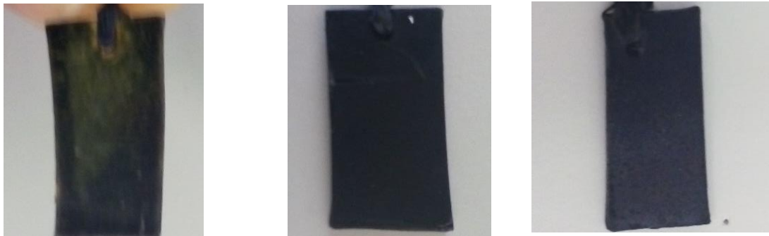
Figure 7. 5-Samples after VPP with PEG (left), pyridine (middle), and after H 2 SO 4 treatment(right)
