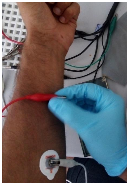
Figure 6. 7 -EIS montage in-vivo . Red wire with PEDOT pin electrode. White wire the AgCl reference electrode
