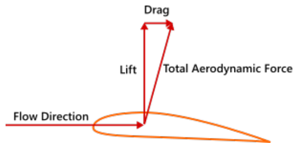
Figure 3.10: Representation of drag and lift on an airfoil
