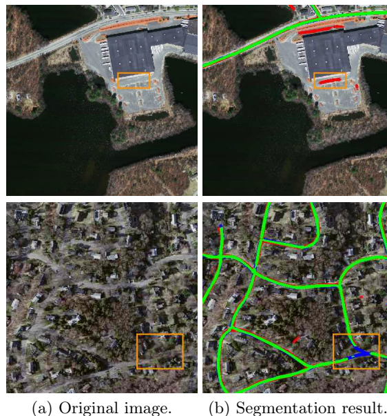
Fig. 1. Illustration of false positives and broken roads (Images taken from Massachusetts dataset [20]). In (b), green represents true positive (TP), red represents false positive (FP), blue represents false negative (FN).
