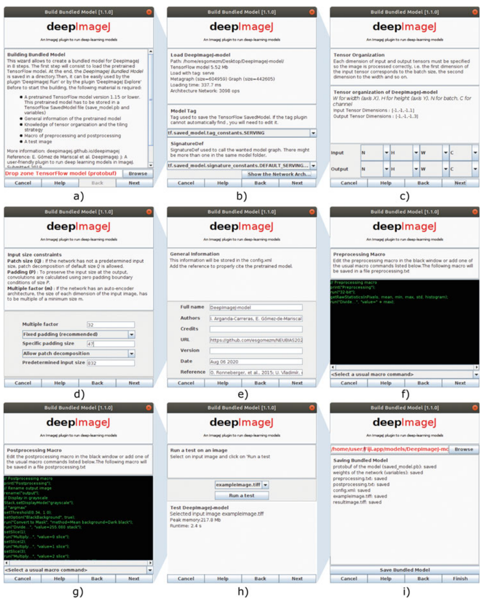
Fig. 4.9 DeepImageJ build bundled model process: (a) Open a test image in Fiji and call Build Bundled Model ; (b) Load a model indicating the path to the unzipped DeepImageJ-model folder; (c) Specify input and output dimension order (N: batch number, H: height, W: width, C: channels); and also (d) input size (32) and padding (47); (e) Write the name of the model, authors, credits, citations or any other relevant information; (f, g) Write the pre- and post-processing macro routines needed for the correct image processing; (h) Run the image processing routine and test that you get the desired output; (i) If so, specify a new name for the bundled model and save it under ImageJ's recently created models folder
