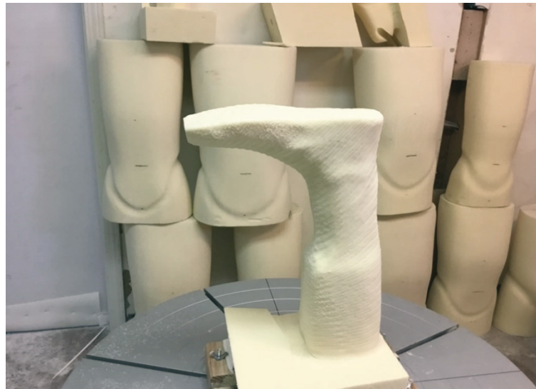
Fig. 2 Moulds for orthoses made using the CAD / CAM technology
