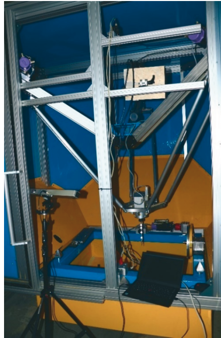
Fig. 7 The vision system follows the markers on the calibration object (tentacle) inserted in the machine tool holder
