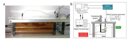
Fig. 1. (a) Experimental apparatus for the measurement of TMMs attenuation coefficient; (b) Experimental set up for the measurement of the temperature increase by means of a fiber optic probe hydrophone.
