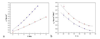
Fig. 2. (a) Attenuation,  $\alpha$ , values and respective uncertainty as a function of the frequency, f, at  $T = (20.3 \pm 0.7)$  °C: • TMM 1, • TMM 2, - fitting curve; (b) Attenuation coefficient,  $\alpha_0$ , values and respective uncertainty as a function of the temperature, T: • TMM 1, • TMM 2, - fitting curve.
