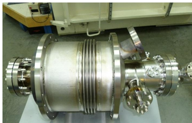
Figure 1: The SRF photoinjector for bERLinPro.
