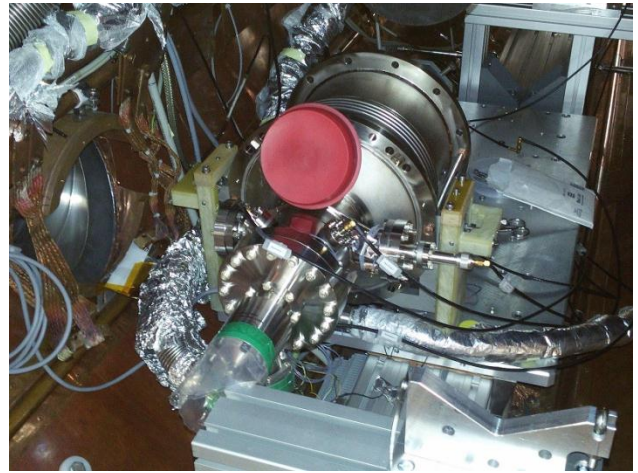
Figure 4: A photo of the gun cavity installed in HoBiCaT.
