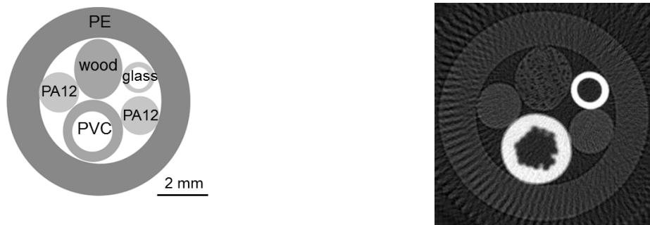
Fig. 7: Sketch of the multi material sample, a PE tube filled with differently absorbing materials (left) and CT reconstruction of the transmission signals at the attenuation detector obtained by filtered back projection ( 3^\circ angular increments).
