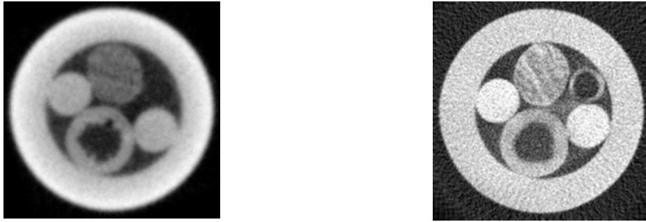
Fig. 11: Reconstruction results obtained from neutron (left) and X-ray Compton (right) tomography. Note that the glass tube is not visible in the neutron result.
