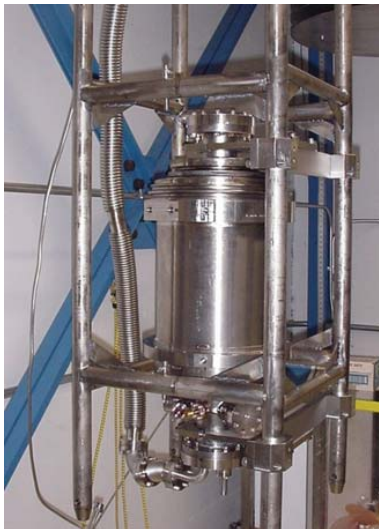
Figure 10: Photograph of the small-grain SRF gun cavity within the He tank at Jlab.
