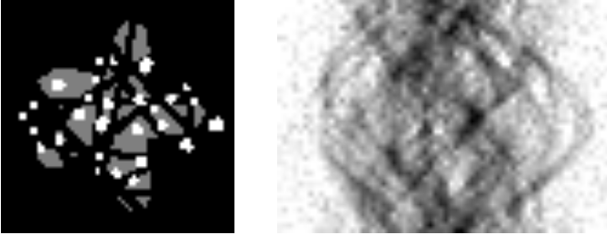
Figure 3: Left: Phantom used for simulation of projections for later reconstruction using the presented algorithm (black: vacuum, grey: carbon black, white: metal). Right: sinogram comprising 45 projections at 4 degrees intervals for the very phantom using a dose of 10^3 counts/pixel.
