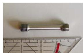
Figure 1: Round tensile test sample with a total length of 60 mm and a gauge length diameter of 6 mm.
