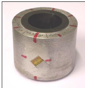
Fig. 1: test specimen consisting of steel insert (S235) and casted aluminium (AlSi9Cu3)
