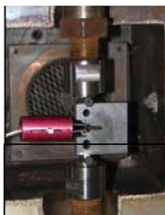
Figure 1. Blunt notch compact-tension specimens are mechanically deformed to generate residual stress (S. Kamel).
