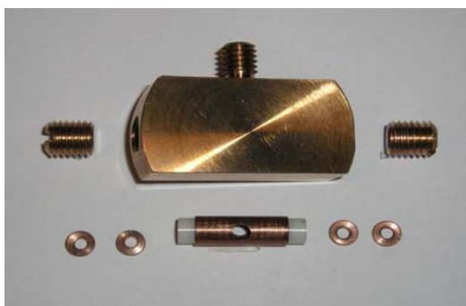
Fig.1 : Uniaxial CuBe pressure cell
