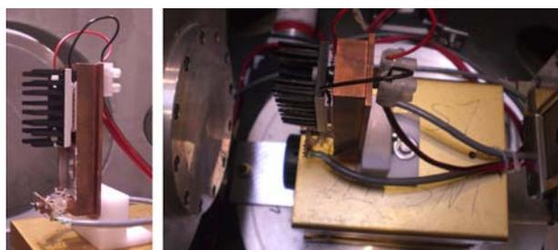
Figure 3: Sample holder consisting of a solid copper block with a Peltier element and PT 100 temperature sensors.
