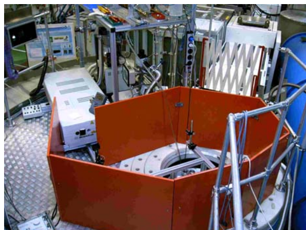
Fig. 1: Optical setup for NEAT, which was developed by us for time-resolved laser-induced experiments.
