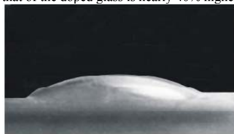
Fig. 2: a) Drop of the pure NCS glass; \alpha=30^\circ
