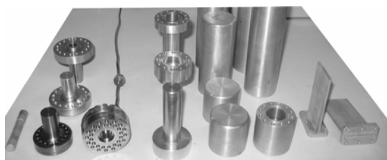
Fig.3: Photograph of available sample containers with different shapes for CGA-OS and CGA-OM.
