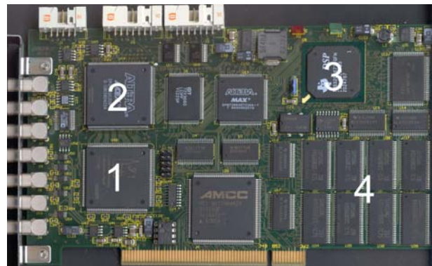
Fig. 1: Front side of the data acquisition board DeLiDAQ , provided with a TDC (1), a FPGA (2), a DSP (3) and a large histogramming memory (4) as main components.
