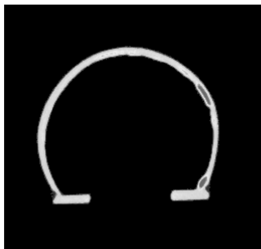
Fig. 2: Pb inclusions inside the brass
