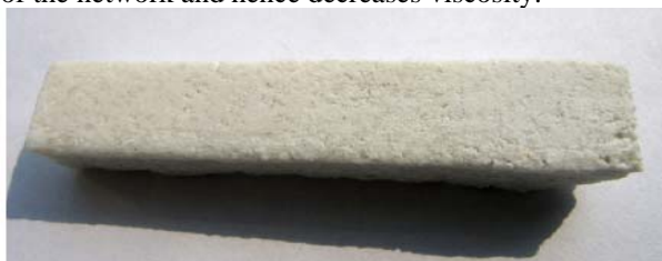
Fig. 1: Nano-scale refractory analogue: Alumina and zirconia nanoparticles embedded in a sodium / potassium silicate glass matrix.
