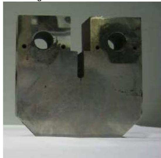
Fig. 1: CT specimen showing crack after heat treatment. Crack is approx 15mm long. Measurements made along the crack.
