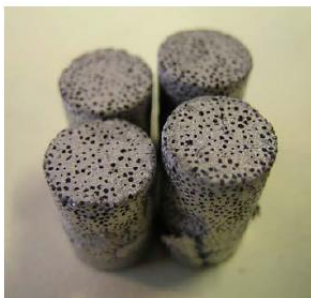
Fig 1: Homogeneous metal-based porous scaffolds (Ti+space-holder)
