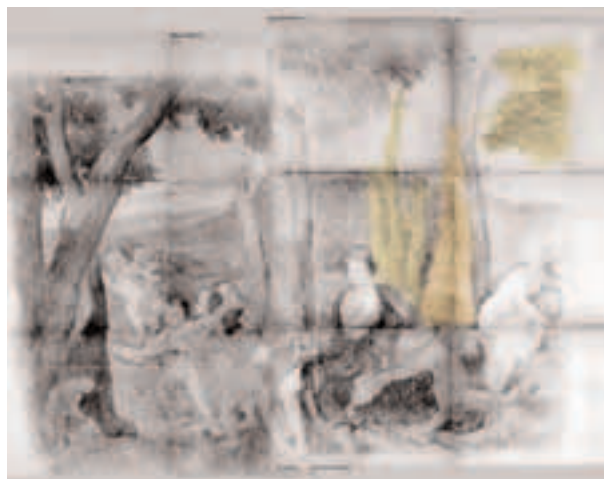
Figure 3. Nicolas Poussin, "Armida abducts the sleeping Rinaldo", 1 st neutron autoradiography assembled from 12 image plate records: In order to investigate the whole picture, two separated irradiations were carried out and finally recombined.
