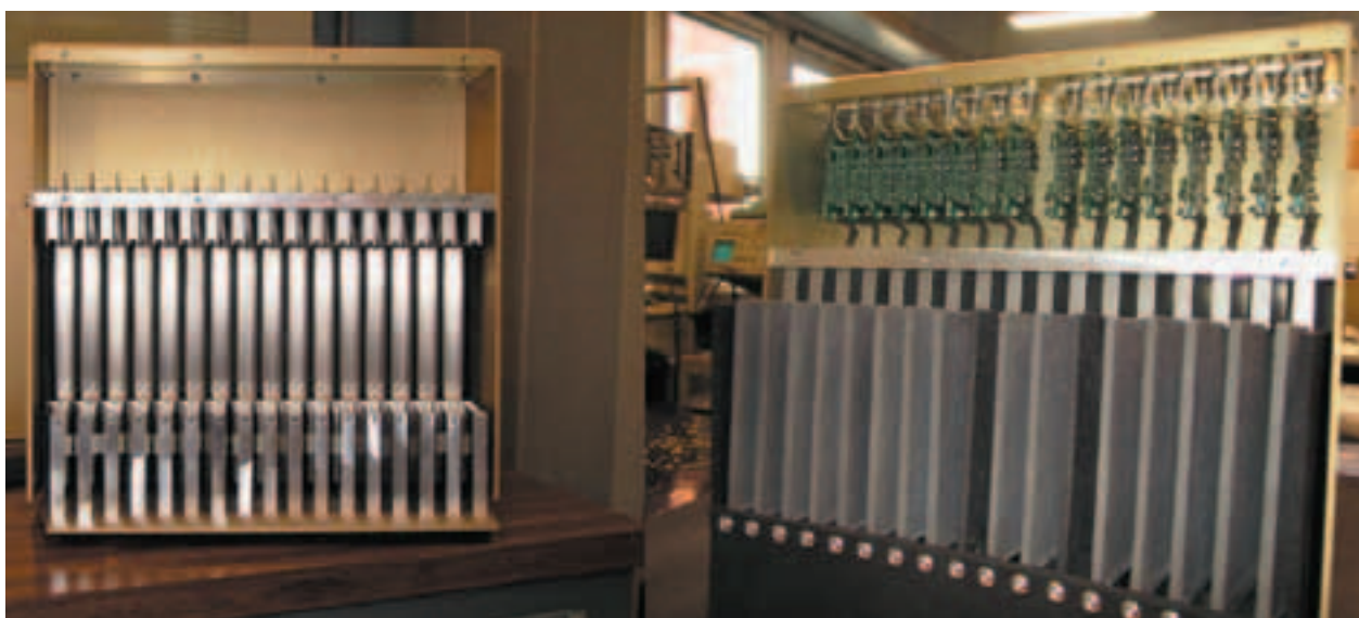
Figure 7. A detector bank is composed of 16 squashed ^3\text{He} tubes ( 100.0 \times 12.5 \times 2.5 \text{ mm}^3 ). The preamplifiers are enclosed in the same box, just above the detectors. The secondary beam collimation is made of \text{B}_4\text{C} ceramic platelets.
