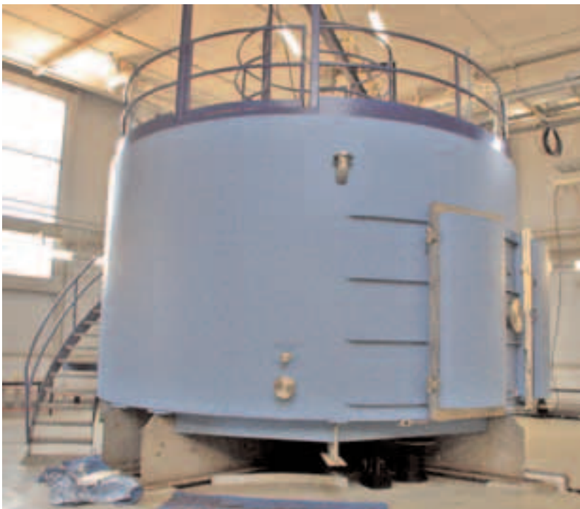
Photo 3. The Backscattering Spectrometer is a near-backscattering, crystal-analyzer spectrometer designed to provide extremely high energy resolution. The design requires a long initial guide section of 84 m from moderator to sample in order to achieve the timing resolution necessary to achieve the desired energy resolution. The tank is 7 m in diameter and 4 m high.
