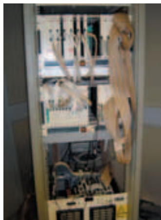
Figure 4. View of the control cabin (left panel) and DAE (data acquisition electronics, right panel). A main computer (actually placed on the desk and connected to the internal ISIS network) is used for controlling the experiment and for data collection.
