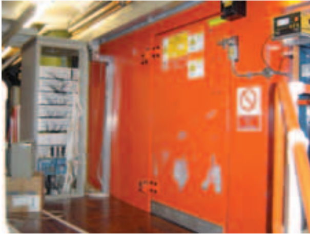
Figure 11. The main door of the INES blockhouse with its radiation control electronics and interlocks. On the left, the electronic rack is visible, that contains the high voltage power supply and the 5 euro-crates with the 80 discriminator cards.
