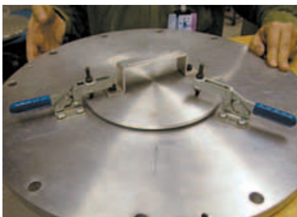
Figure 6. A reduced vacuum flange is available for routine room temperature experiments.
