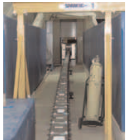
Photo 5. This curved portion of the 84 m of neutron guides directs low energy neutrons from the target to the sample. Photo credits: ORNL
