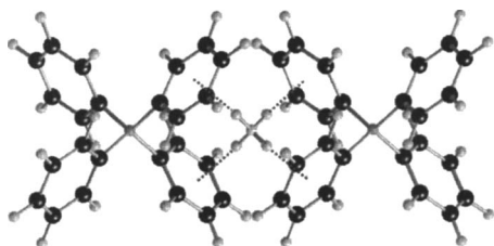
FIG. 1. The structure of ATPB determined by neutron diffraction (Ref. 3). The ammonium ion is located between two tetraphenylborate cations. Each of the N^+-H\cdots Ph interactions can form an aromatic H bond (indicated by dashed lines in the center of the figure).
