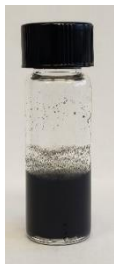
Figure 4.6: Image of \text{Ti}_3\text{C}_2\text{-PEG6} dispersed in \text{H}_2\text{O} at a concentration of \sim 1 mg/mL. The lingering flakes above the solution occur due to residual immiscible chloroform post reaction solvent exchange back to water.
