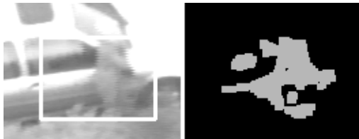
Fig. 5. A poorly segmented pedestrian. Whichever match matrix is chosen for the reference standard, the result will always be unsatisfactory
