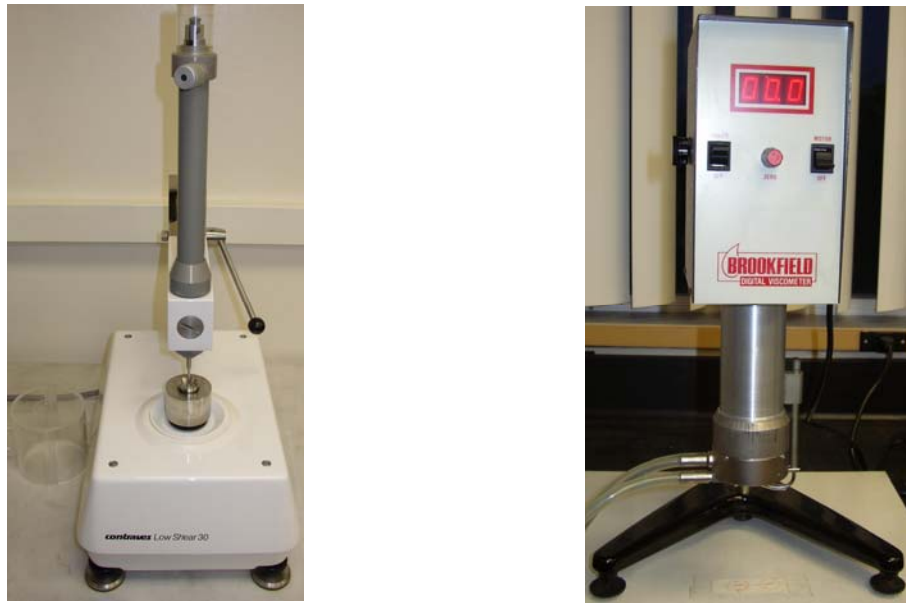
Figure 5.1.2: The most widely used rotational viscometer systems: Contraves LS-30 (left photo) and Wells-Brookfield (right picture).
