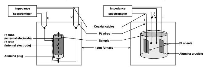
Sample dimensions: I = 3.5 to 9mm od = 4.5 to 7.5mm id = 1mm
