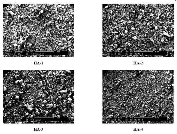
**Fig. 2.** SEM micrographs of freeze-dried HA (magnification level of  $25 \times$ ).
