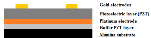
Figure 1: Schematic representation of thick-film structure.
