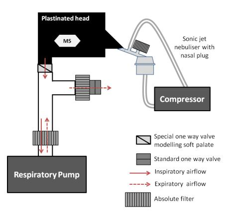
Figure 1: Schematical experimental set-up for nebulization simulating an inspiration by the nose and exhalation trough the mouth thanks to the respiratory pump.
