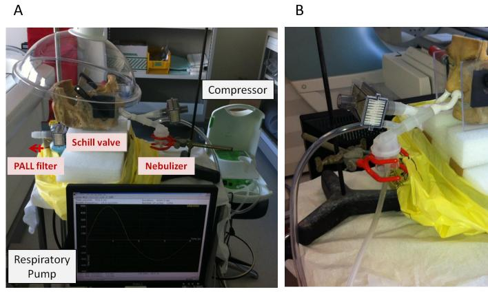
Supplementary Information: Experimental set-up for nebulization. A and B corresponds to photography of the set-up in the Nuclear Medicin department (CHU Saint-Etienne).
